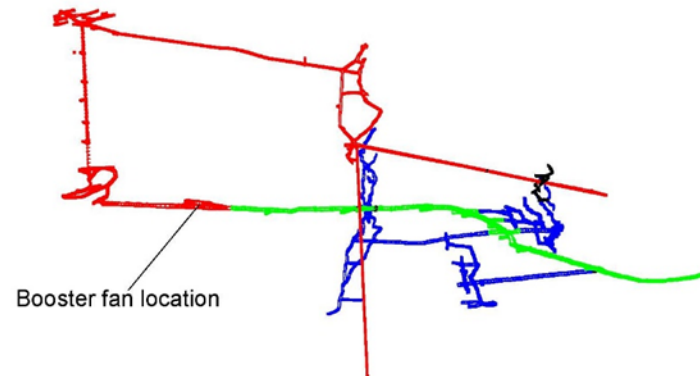
Figure 16-2: Ventilation layout of the Velardeña mine
