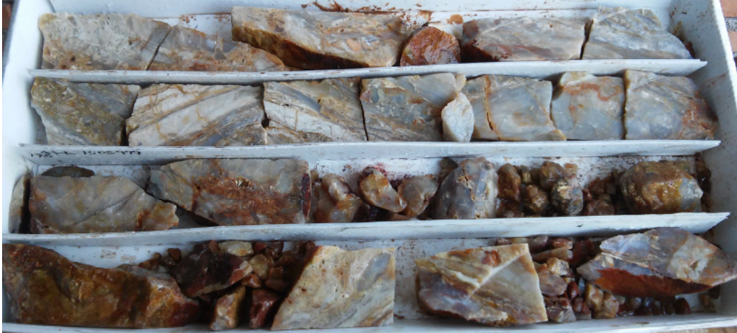
Figure 10-1: Typical Drill Hole Recovery and RQD (RDO16-07 17 m)
